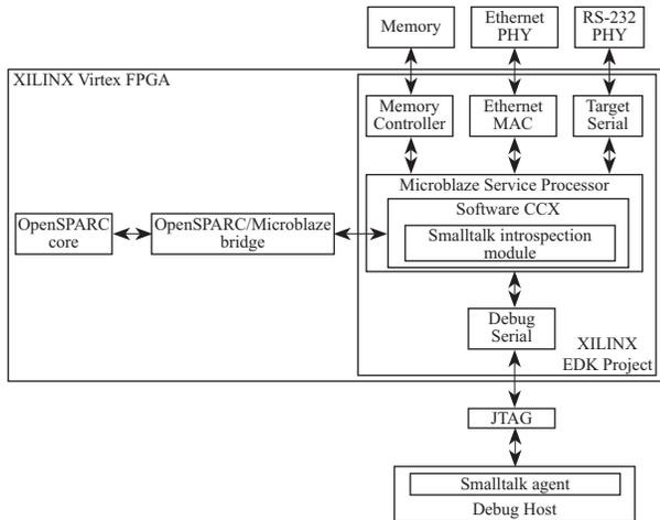
**Figure 3.** OpenSPARC Implementation on XILINX Virtex FPGA with Smalltalk-Aware Crossbar. Cf. the corresponding diagram in [Thatcher’08], NB the position of the Smalltalk module.
